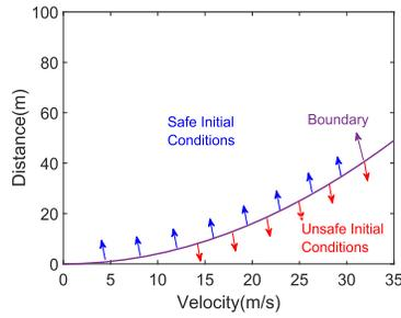
Fig. 8. Safe initial conditions for full braking action.
