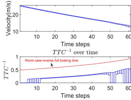
Fig. 13. The inverse TTC over time is smaller than the worst case inverse full braking time  $\tau^{-1}(\max(v))$ . The AEBS is safe (for 60 time steps) with the initial conditions  $d_0 \in [97, 97.5]$ ,  $v_0 \in [25.2, 25.5]$ .
